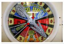
STEP # 2: Using the 7/64 Allen Wrench, remove the two allen bolts that hold the ghost arrow to the pulley
