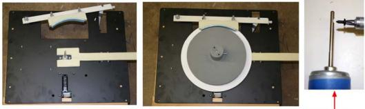
NOTE: UNITS BUILT AFTER 3/01/07 HAVE A NOTCH CUT INTO THE MOTOR SHAFT THAT THE SET SCREW TIGHTENS INTO. IF YOUR UNIT IS DATED AFTER 03/01/07 - THE SET SCREW MUST BE BE TIGHTENED INTO THIS NOTCH TO FUNCTION.
